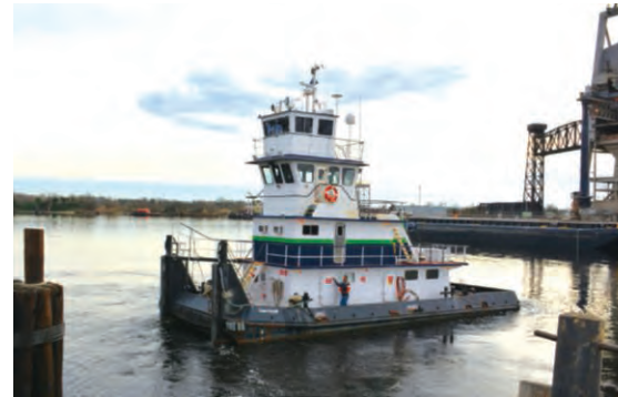
The 55-foot-long, 1,500-horsepower tugboat Chatham heads out from Vane's Paradise Creek location.
