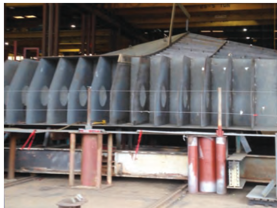
The stern of the first AT/B hull is turned upside down as construction takes place in early March.
