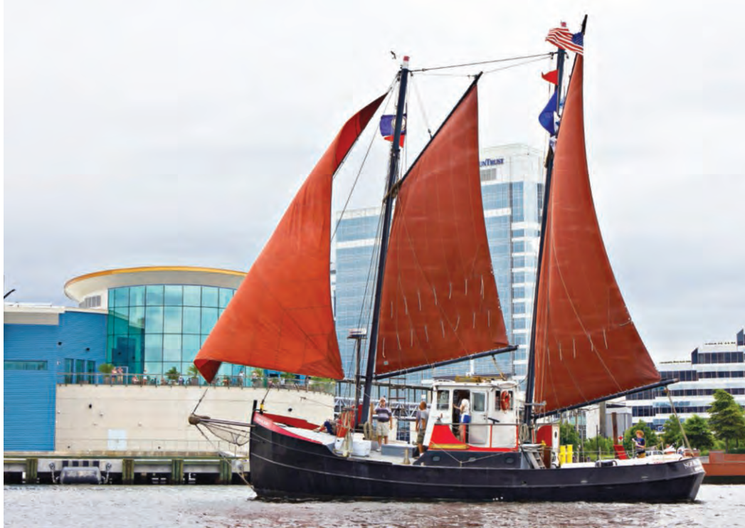
The Norfolk Rebel , launched in 1980, is possibly the world’s only sail-assisted, schooner-rigged tugboat.
